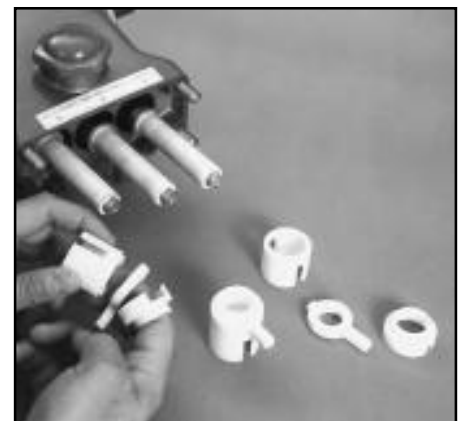
Removal of Seal Retainers and Wicks
