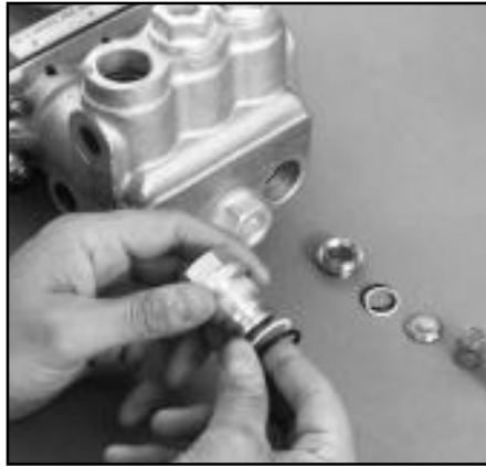
Examination of O-Ring and Back-up-Ring on Valve Plug
