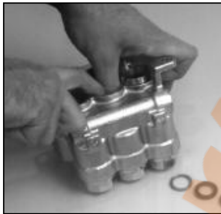
Installation of Male Adapter
