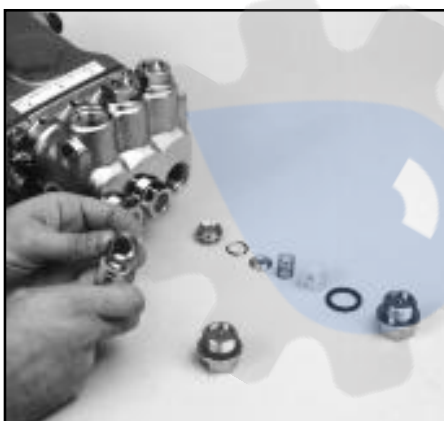
Order of parts in Valve Assembly
